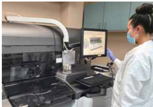
Tiffany Belgarde, MLS, in the Mobridge Regional Hospital & Clinics Laboratory Department, works with the new Vitros 7600 chemistry analyzer.
